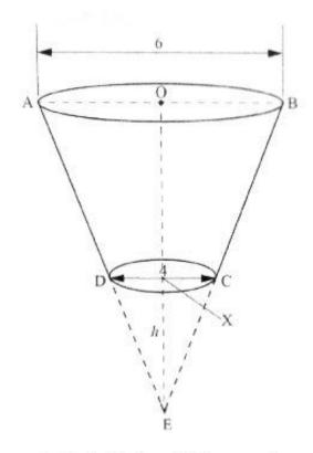
The diagram above shows a tumbler in the form of a frustrum of a cone ABCD with base diameter of 4cm, top diameter of 6cm and a height OX of 12 cm. O is the centre of the top circle and X is the centre of the bottom circle. E is the vertex of the cone where XE = h cm.
